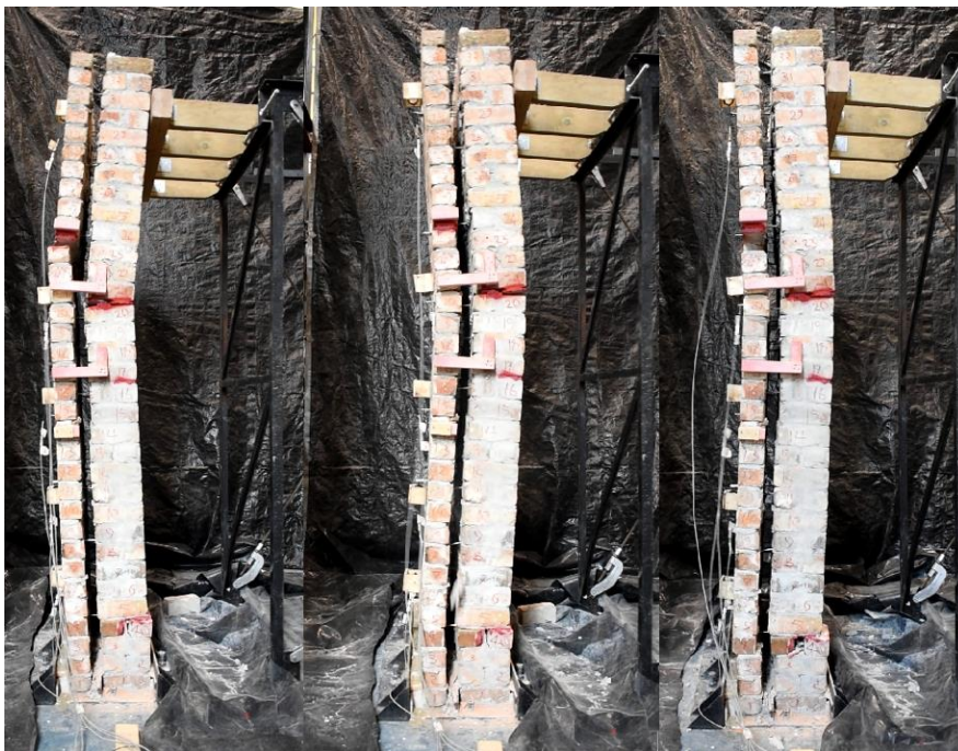
Figure 12: Wall W6: stills from video record of testing showing rocking behaviour
