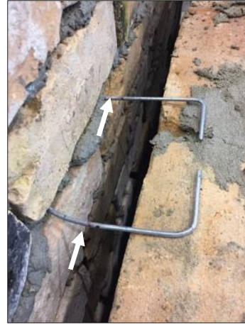
(b) Notched wire hoop simulating historical as-built ties.
