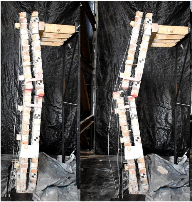
Figure 9: Wall W5, stills from video record of testing showing rocking behaviour and collapse
